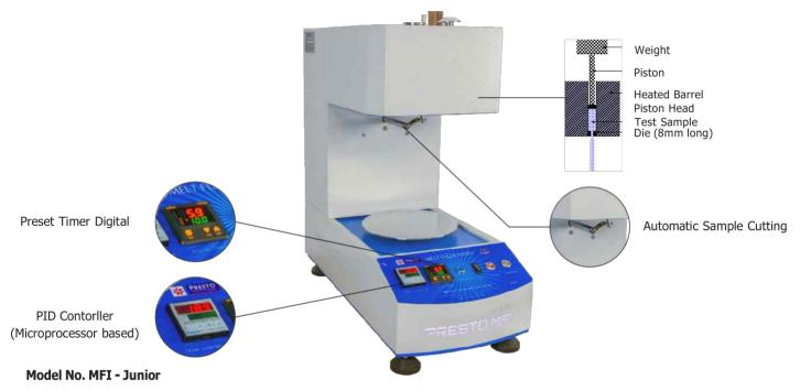
**Melt Flow Index Tester** is a consistent tool useful for checking the flow properties of molten plastics/resins. PRESTO Melt Flow Index Tester is manufactured under various Test Standards ASTM D 1238-1992, IS 2267-1972, IS 2530-1963, IS 10810-1984.
